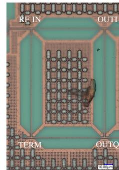
Fig. 7: Micrograph of reduced-size branch-line quadrature hybrid.
