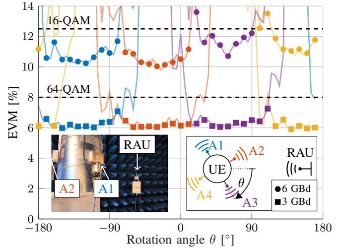
Fig. 4. Self-blocking problem resolved: Measurement of spatial diversity at user equipment (UE) ensures 24 Gbps (6 GBd) or 18 Gbps (3 GBd) over 360° by combining signals at Antennas 1, 2, 3 and 4 (A1, A2, A3 & A4).
